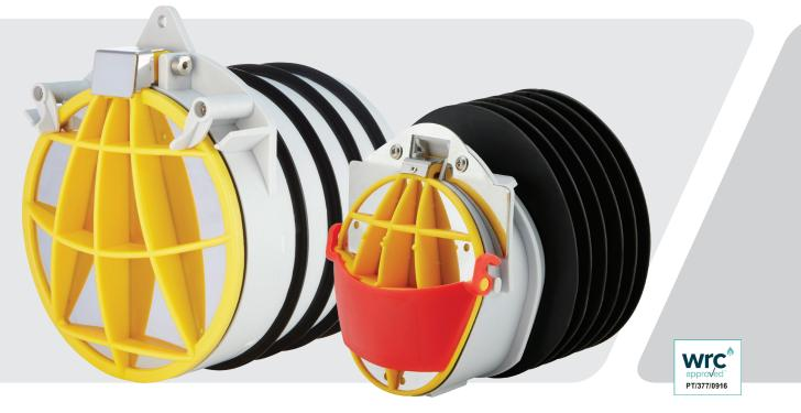
Flexseal's range of retrofit Non-Return Valves (NRV's) can be installed directly into existing manholes by simply pushing the NRV into the desired pipe inlet. The product prevents foul water flowing back from the blocked sewerage systems to flood the property from the inside via toilets, plug holes and waste pipes.
